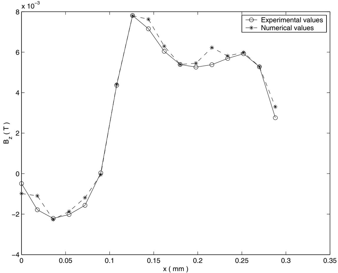
**Numerical values of  $\mu H_z$  with  $M = 55$ ,  $N_{\text{total}} = 16,152,290$ ,  $\eta_{\text{total}} = 0.0105$ , the number of degrees of freedom on  $\mathcal{T}_M$  is 120,558.**
