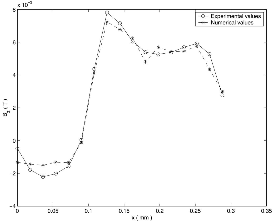
**Numerical values of  $\mu H_z$  with  $M = 55$ ,  $N_{\text{total}} = 5,555,550$ ,  $\eta_{\text{total}} = 0.0126$ , the number of degrees of freedom on  $\mathcal{T}_M$  is 36,714.**
