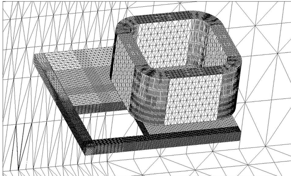
An adaptively refined mesh of 2,263,668 elements after 18 adaptive iterations from 77,760 initial elements.
