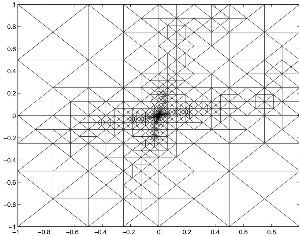
**The adaptive mesh of 2673 nodes. The energy error is 0.07451.**
