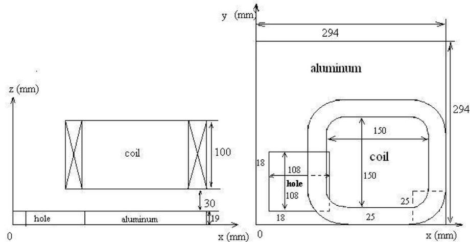
**Team Workshop Problem 7.** This problem consists of an aluminum plate with a hole above which a racetrack shaped coil is placed. The aluminum plate has a conductivity of  $3.526 \times 10^7$  Siemens/Metre and the sinal driving current of the coil is 2742 Ampere/Turn. The frequency of the driving current is  $\omega = 50$  Hertz.
